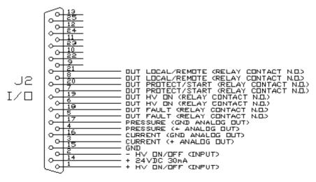
CURRENT LOGARITHMIC OUTPUT : 0V=100mA ; 6V=100mA PRESSURE LOGARITHMIC OUTPUT : RELAY CONTACT : 24V 100mA
